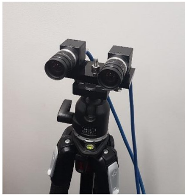
(a) Our stereoscope, fitted with the 75 mm base plate
